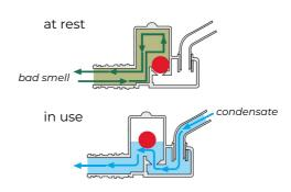
Reversible condensate drain wall box. Pipe connector ø 16-18 and ø 18-20 with o-ring.
